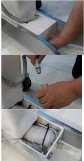
Image 2: Remove the cover plate by pulling.
