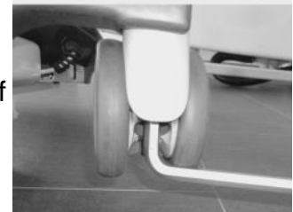
Image 4: Unscrew the screw of the castor using the Allen wrench.
