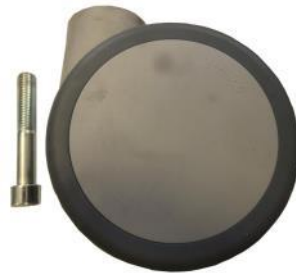
Image 5: Remove the screw of the castor. Hold the castor back with your hand! Remove the castor with the screw
