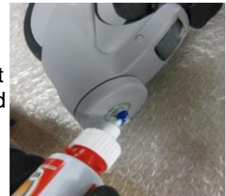
Image 6: Prior to screwing a new castor, you must apply thread lock fluid (medium tight at least 21 Nm) to the thread of the screw.
