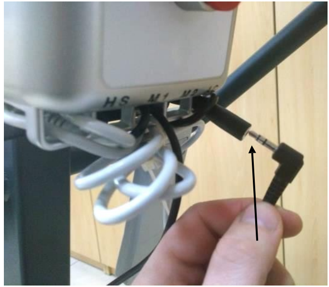
Figure 22 – Connecting the charging cable
