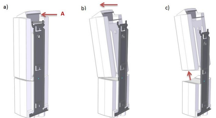
Figure 21 – Battery removing (A – release lever)
