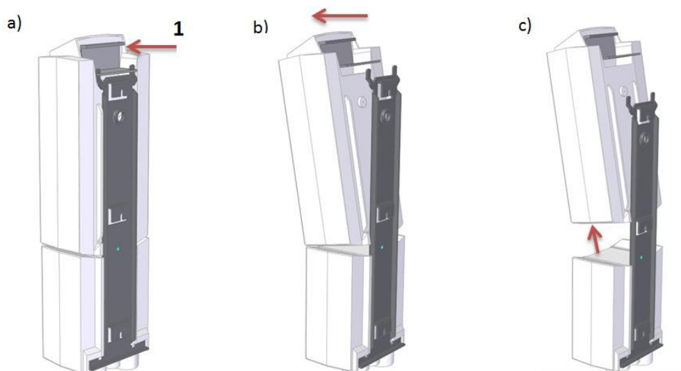
Figure 13 – Battery removing (1 – release lever)
