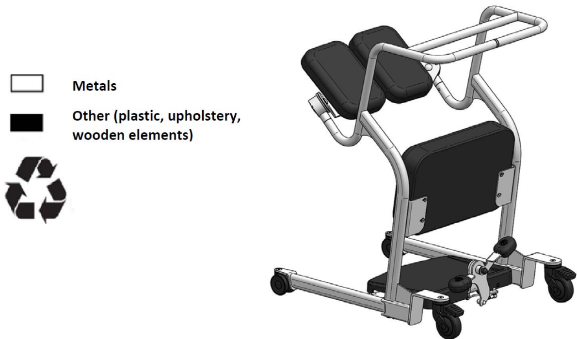
Figure 6 – Recycling the Elevand SteadyStand mobile patient lift
