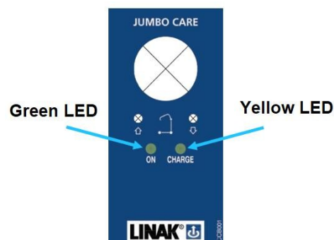
Figure 25 – LED location on the control box
