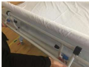
Fig. 5.2 – " Working-position " (during turning) the roll in one side is turned from the bottom position to the top position
