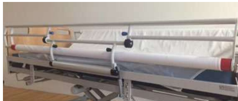
Fig. 5.1 – " Bed-rail position " (during turning) one side has the roll on top and the other side operate as bed rail
