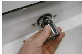
Figure 18: Switch off the solenoid valve.
