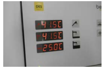
Figure 16: The picture shows the desired maximum temperature, which must agree with the manually measured temperature.
