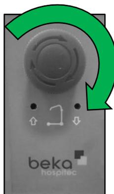
The emergency stop switch is released by turning the button to the right (i.e. clockwise).
