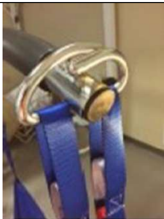
Sling loop correctly positioned at the base of the carry bar hook.
