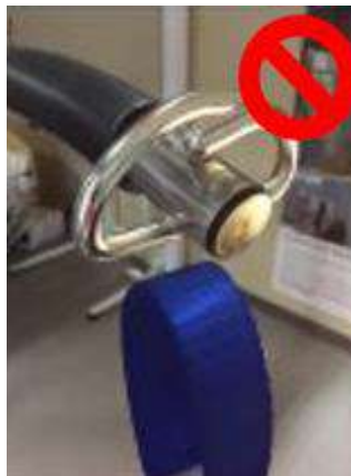
Sling loop separated from the carry bar hook.
