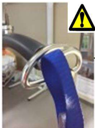
Load applied. The sling loop begins to slide off the hook.
