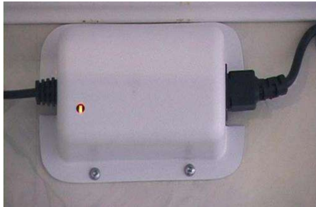
Charger with ORANGE light indicating that the lift is connected and charging. When the lift is fully charged this light will turn GREEN .
