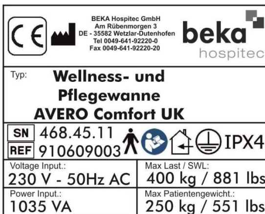
Picture 4 Illustration shows the type label. The type plate is placed on the side of the pult. The shown serial number 468.45.11 is an example. Please indicate in case of questions always the serial number of the type plate of your device.
